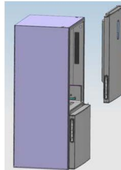
2. a. Screw off the 3 screws of the middle hinge cover, and then remove the middle hinge.
