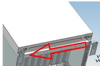
b. Assemble the shorter adjustable front foot to the lower hinge side, and adjust the height of the foot to make the refrigerator level.
