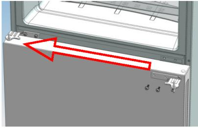
3. Install the fridge door, assemble the left upper hinge to the other side of the cabinet, and use a tool to screw up the 4 screws to fix the upper hinge. Then, connect the door communication wire and the cabinet communication wire, install the left upper hinge cover, and fix it using a screw.
