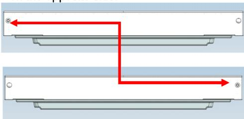
b. Screw off the screws of the stopper as shown below, and assemble them to the other side of the door.
