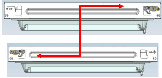
c. Remove the axle and two stoppers on the lower hinge, and assemble them to the position as shown below.
